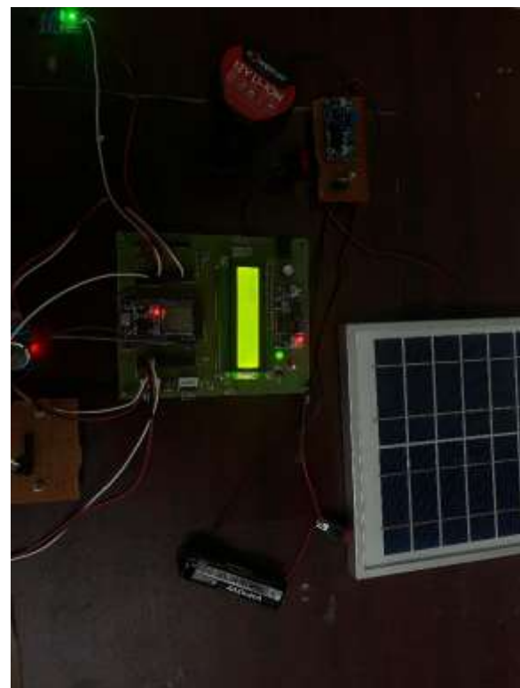
Figure 2 The hardware prototype of the proposed IoT-enabled smart perimeter security fence system
